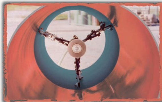
Air-motor controlled adjustable carriage legs quickly center the paint head within the pipe.
