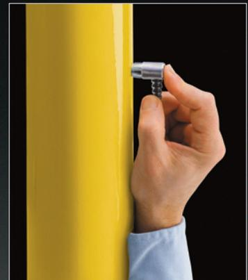
**UTG M Thru-Paint models** measure the metal thickness of a painted structure without having to remove the coating.
